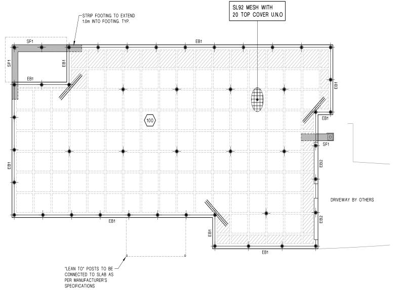
FOOTING & SLAB PLAN SCALE 1:100
