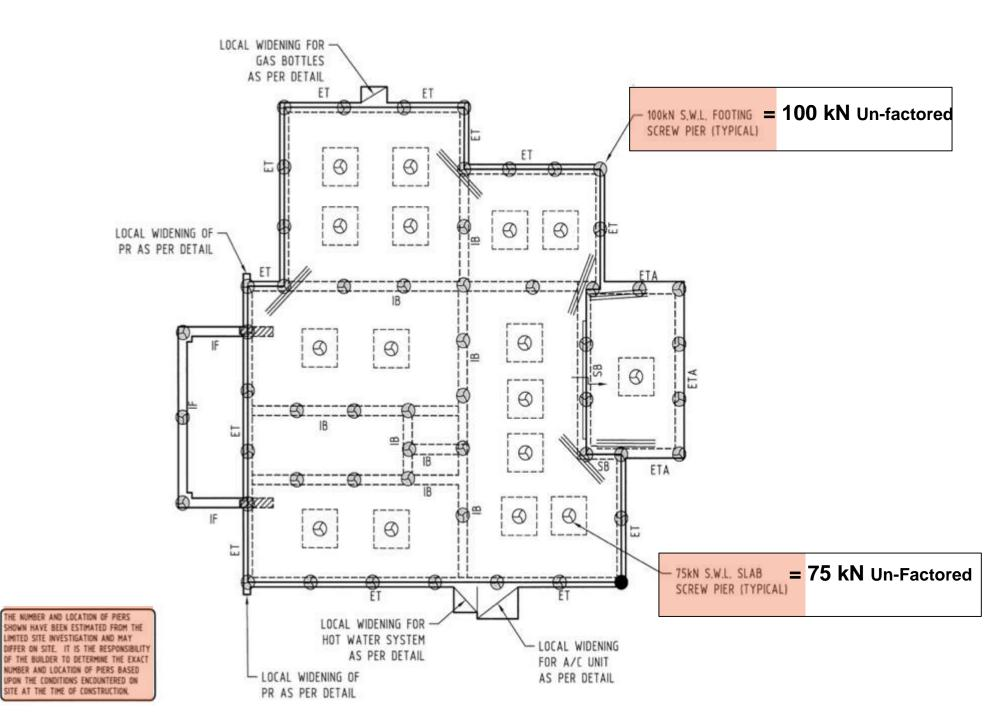
Providing the wrong pile loads for each location, means the client pays for piles that they don't need
