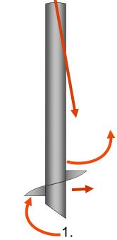
Screw piles have one leading edge with a curved pitched helix that augers the soil during install. The single leading edge induces out of round forces.
