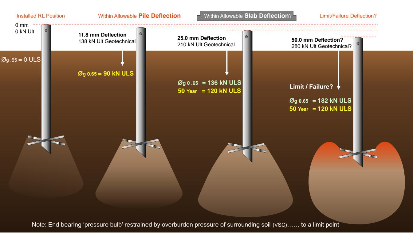
Øg allowed solely from 'on site' AS2159 static load pile testing - 1.0% = 0.55, 2.0% = 0.65, 3.0% = 0.71, 4.0% = 0.76 (% of total piles).
